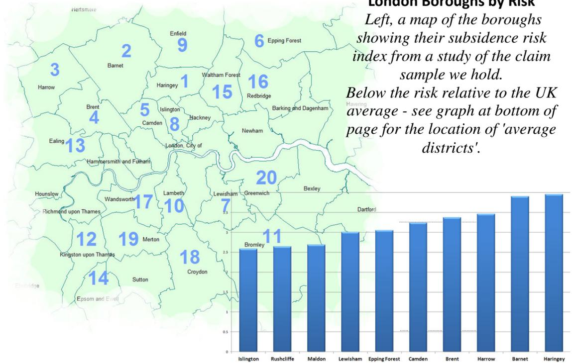
The above map and graph have been produced from a claim sample of 103,000 records plotting claims divided by housing population per borough. The graph plots the output by the 'times riskier than the UK average'. For example Harrow is 3.5 x riskier, and Islington 2.6 x riskier than the UK average. Haringey is top of the table with a value 4 x greater than the UK average.
